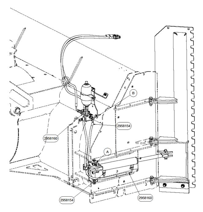
A: The bracket for the cylinder must be installed as in the illustration. B: 2 pcs. holes threaded M10.
